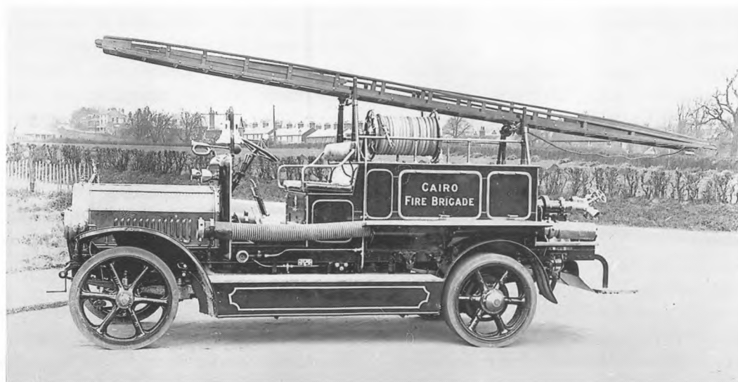
Fig 16.7 Dennis fire engine manufactured for the Cairo Fire Brigade, 1920. Reproduced by permission of Surrey History Service (1463/PHTALB/1/3 f.77)
